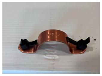
**Step 4:** Take a second zip tie and slide it down the first zip tie you already inserted to secure the clamp tightly to the launcher. Cut off any extra plastic. Repeat this process on the other side of the clamp to fully secure it.
