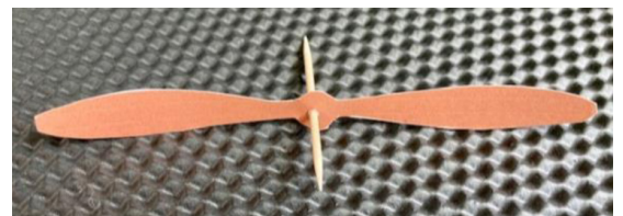
Figure 5. Push the toothpick through the hole in the center of one of the rotor blades
